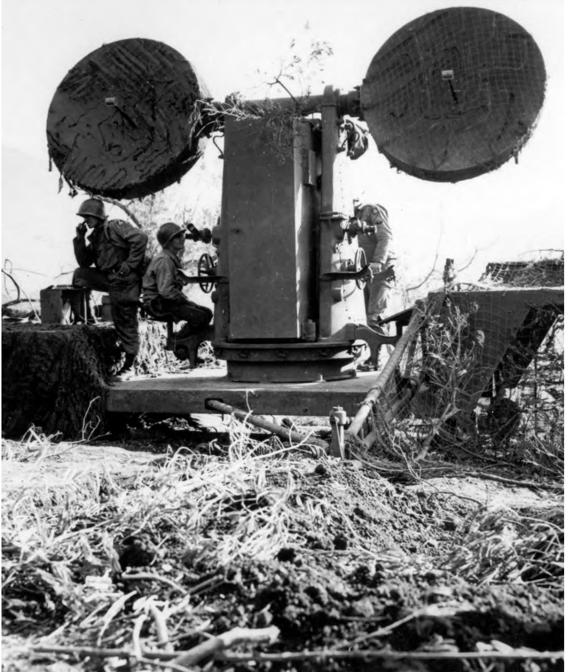
RADAR IN OPERATION NEAR SAN PIETRO INFINE. The operating parts were mounted on a semitrailer towed by a tractor or truck. A van-body truck carried a complete stock of spare parts. (Radar SCR 547.)
