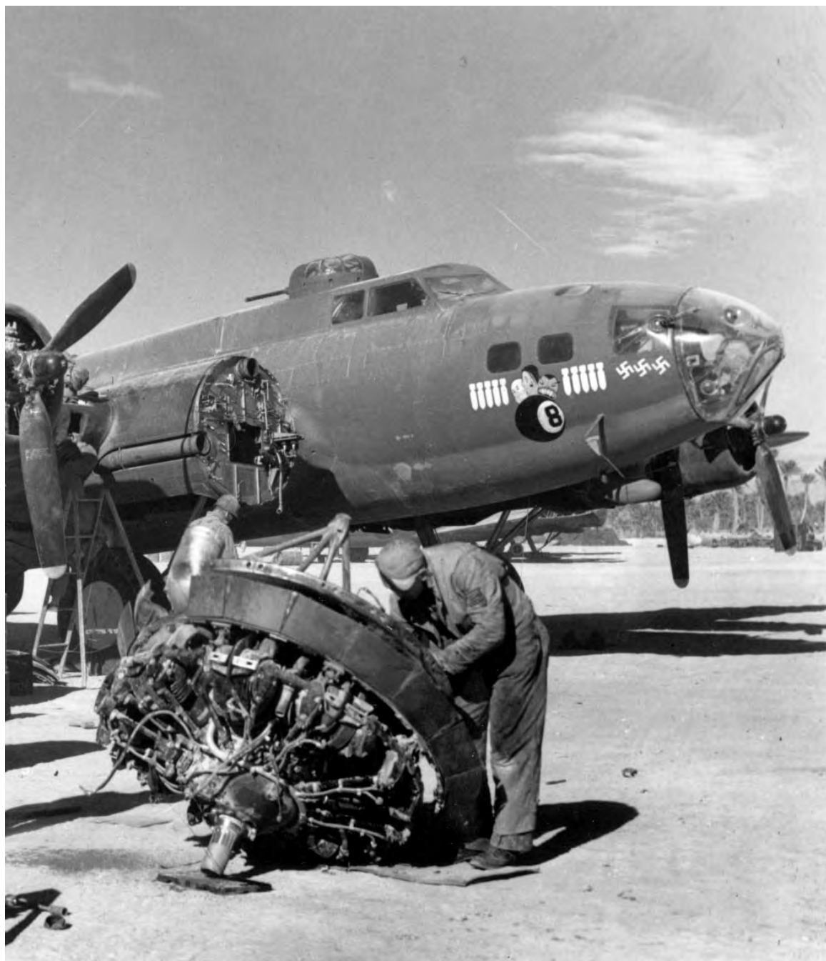
REPAIRING MOTOR OF A HEAVY BOMBER, the Boeing Flying Fortress. The sand and dust of the desert were hard on engines of all kinds. On the nose of the plane, swastikas indicate number of enemy aircraft shot down and bombs show number of bombing missions flown. (B-17.)
