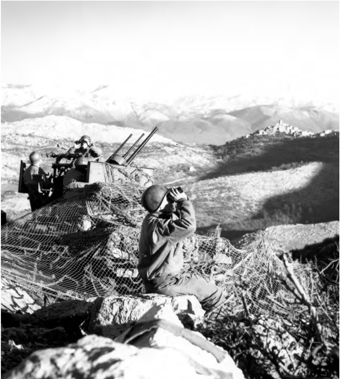
CAMOUFLAGED MOBILE ANTI-AIRCRAFT UNIT near San Pietro Infine. Enemy air attacks were not very numerous during the Winter Line fight; the Germans had few aircraft to spare and the weather tended to restrict the use of enemy as well as Allied aircraft. (Multiple-gun motor carriage M15 composed mainly of a half-track personnel carrier with a 37-mm. gun, two .50-caliber machine guns, and M6 sighting system.)
