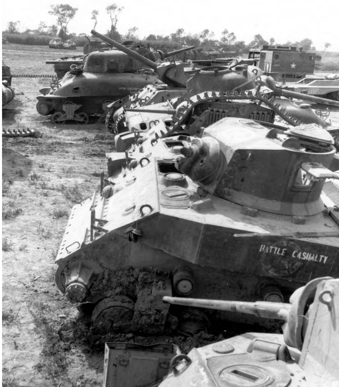
A GROUP OF ARMORED VEHICLES at a salvage yard of a heavy maintenance company in Italy. (1, 2, and 3, light tanks M5; 4, medium tank M4; 5, gun motor carriage M10; 6, medium tank M4. A tractor and tank recovery trailer are partially visible, upper right.)
