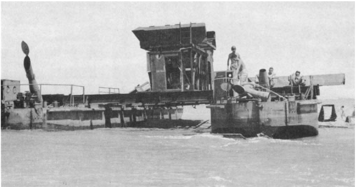
GERMAN SIEBEL FERRIES. These diesel-powered, ponton-raft ferries were used to transport supplies from Italy and Sicily. They usually traveled in convoys and were often heavily armed with 88-mm. anti-aircraft guns when moving toward Tunisia as well as with the lighter protection which they retained for the return trip. Of shallow draft, they could unload directly onto the beach, a factor which became especially important after the Allies had gained control of the air and subjected the Tunisian ports to severe bombing.
