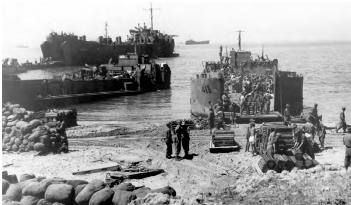
LANDING CRAFT ON BEACH. Top picture from left to right: LCI, LCM, and LCVP; on beach is a 1/4-ton 4 x 4 truck, jeep. Bottom picture: in middle distance is LST, with bow doors open, ramp down, and unloading onto a sectional ponton ramp; in the foreground are two LCT's. (The LCI (L) (1-350) was an infantry carrier with side ramps which could be lowered for unloading directly on the beach. It carried a crew of 3 officers and 21 men.)
