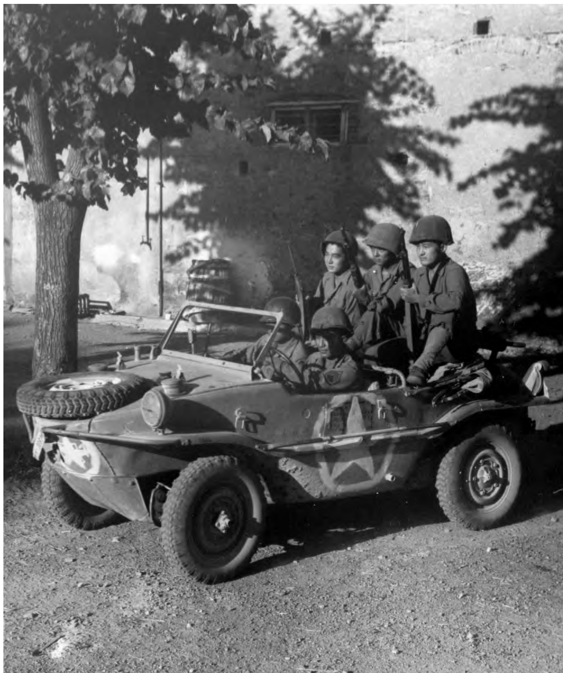
GERMAN AMPHIBIAN JEEP, a version of the light Army car, Volkswagen. Both versions were inferior in every respect to the U. S. jeep except in the comfort of the seating accommodations. ( Schwimmwagen, 1e.P.Kw.K.2s. )
