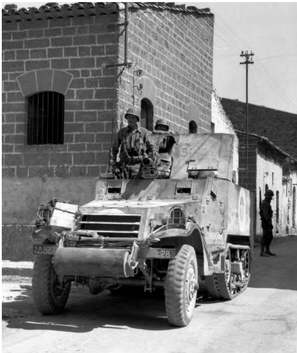
HALF-TRACK MOVING THROUGH A SICILIAN TOWN. The gun is a 75-mm. howitzer M1A1 used generally as an infantry support weapon. (75-mm. howitzer motor carriage T30.)
