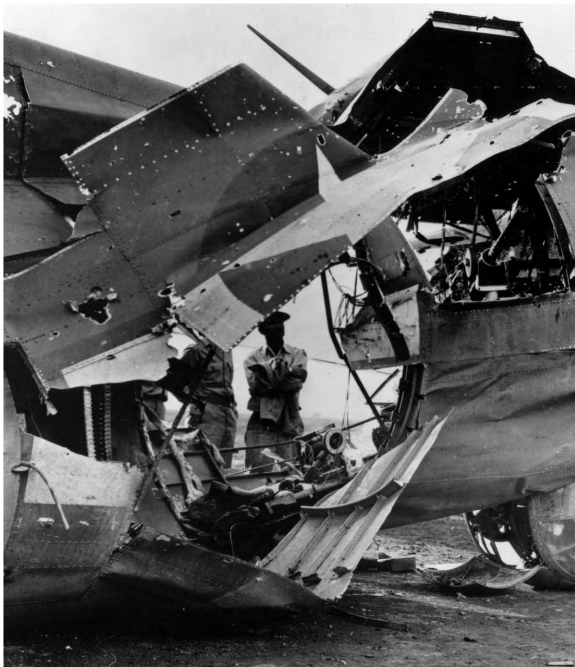
FLAK-DAMAGED FUSELAGE OF A FLYING FORTRESS. This plane received a direct anti-aircraft shell hit while on a mission over Hungary but managed to fly back to Italy where it collapsed on landing. In spite of damage to the bomber none of the crew was hurt.
