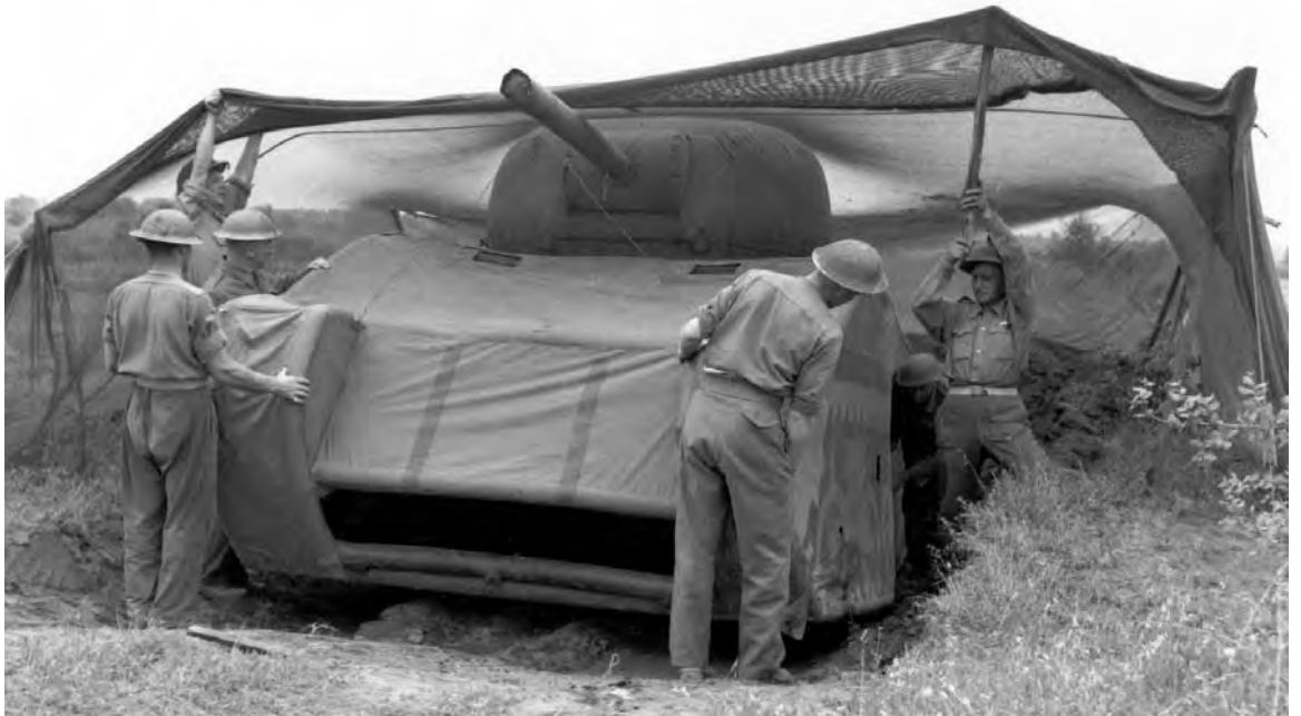
INFLATING RUBBER DUMMY TANK (top). Placing dummy tank in camouflaged position which had been vacated by a tank moving toward the front for the coming offensive (bottom). The dummy tank was designed by the British and manufactured in the United States.
