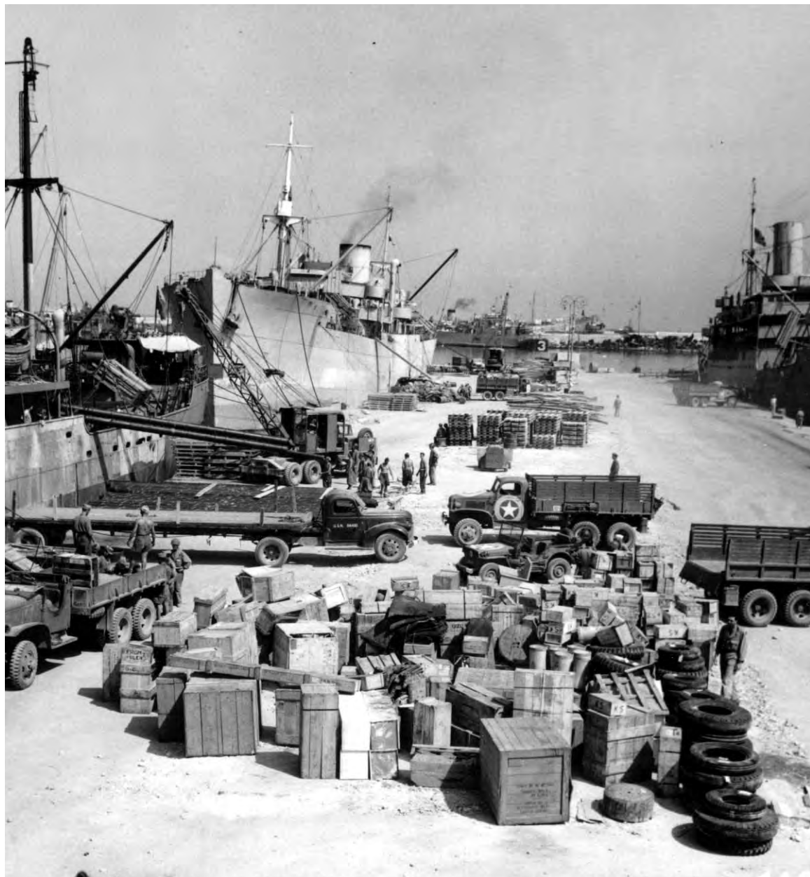
UNLOADING EQUIPMENT IN PALERMO. Even before the fighting in Sicily had ended, the build-up for the invasion of Italy started. The crane (left center) unloading pipe is a truck-mounted crane M2. Designed to handle 240-mm. howitzer materiel and 8-inch gun materiel in the field, it was a six-wheeled type with power supplied to all wheels and capable of accompanying convoy vehicles at a maximum speed of about thirty miles per hour. It was also used to facilitate unloading as above. The crew consisted of a chassis operator and a crane operator.
