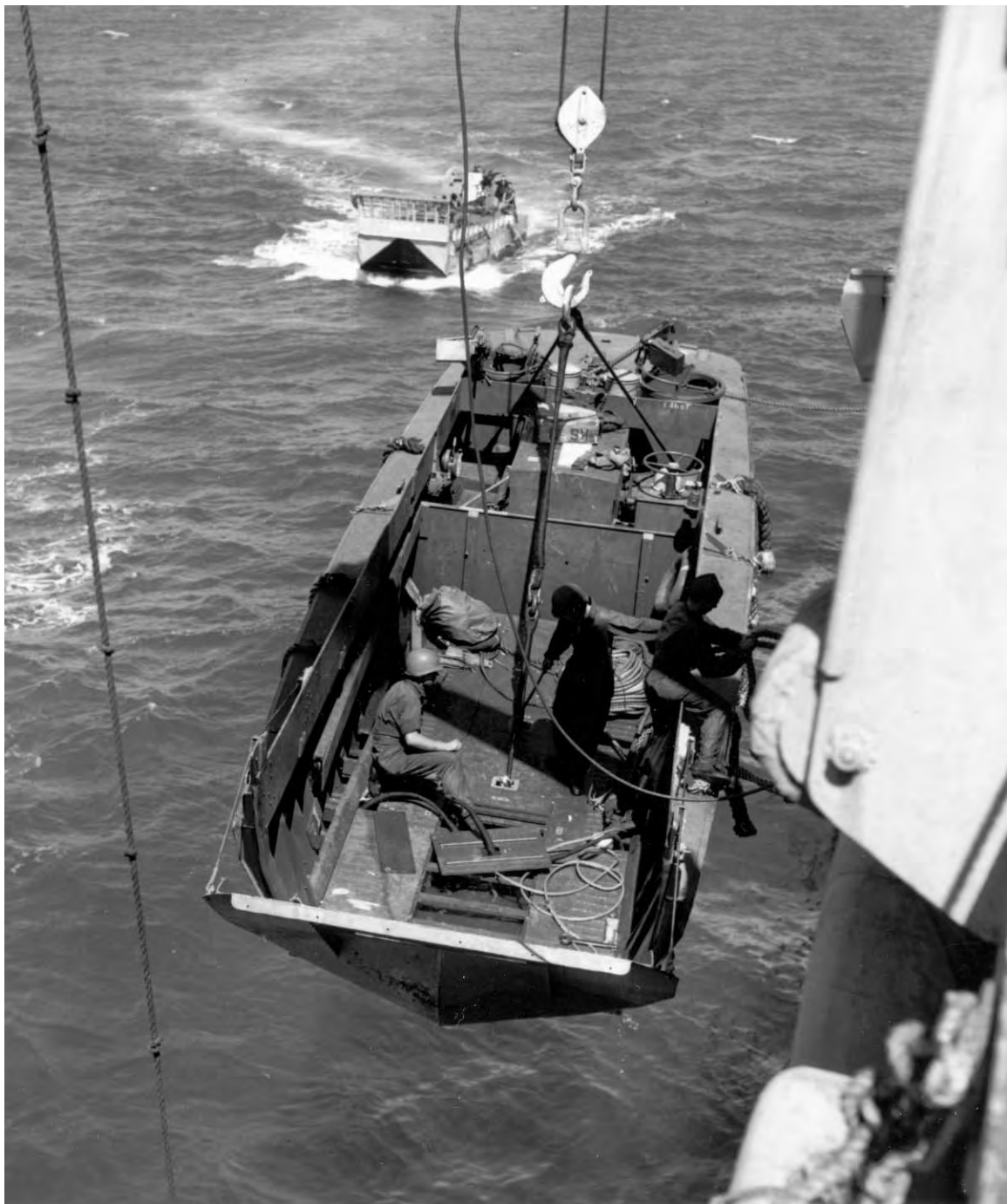
LOWERING LANDING CRAFT OFF GELA BEACH. Troops boarded the craft after it was afloat. (Foreground, landing craft, vehicle-personnel, LCVP; background, LCM.)
