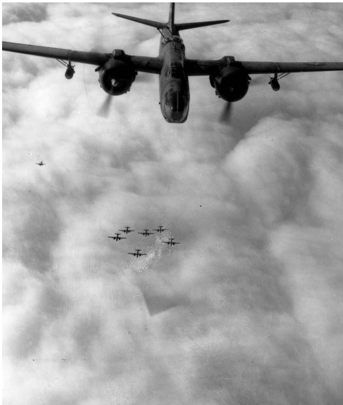
LIGHT BOMBER, DOUGLAS A-20. This was a fast, versatile, and heavily armed plane used for both bombing and strafing in Tunisia. The American version was usually called the Havoc and the British version, the Boston.
