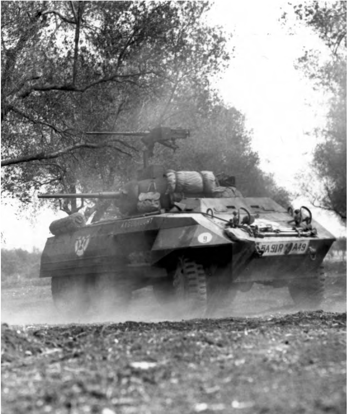
ARMORED CAR FIRING ITS CANNON IN THE CASSINO AREA. (Armored car M8; principal weapon, 37-mm. gun. The one above is also equipped with a .50-caliber M2 Browning machine gun in AA mount.)
