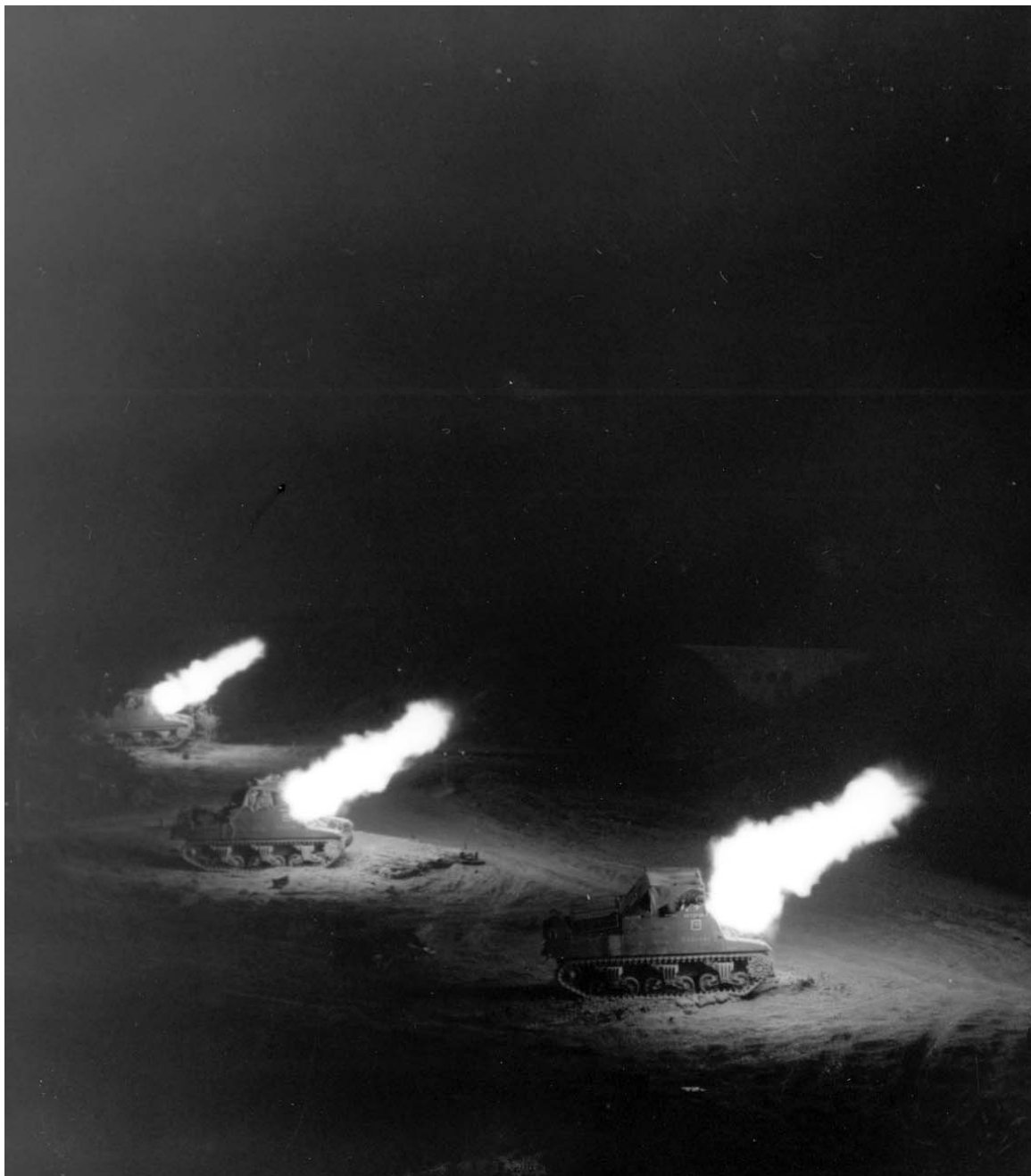
SELF-PROPELLED GUNS of a South African armored unit firing a mission a few days before the attack to break into the Po Valley. These vehicles are American Sherman tanks modified by the British as self-propelled guns. Prior to the jump-off, the units along the Fifth Army front had been engaged in a series of deceptive artillery fires.
