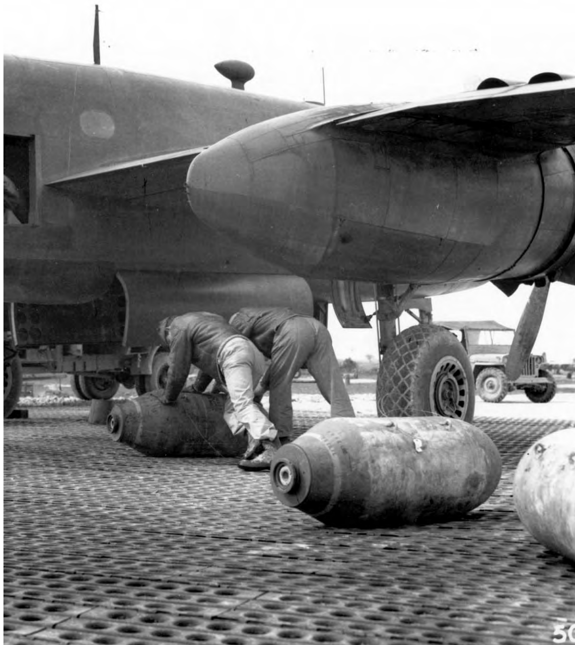
LOADING A MITCHELL MEDIUM BOMBER, North American B-25, with 1,000-pound bombs. Tail fins were attached to the bombs after they were in position in the bomb bay.
