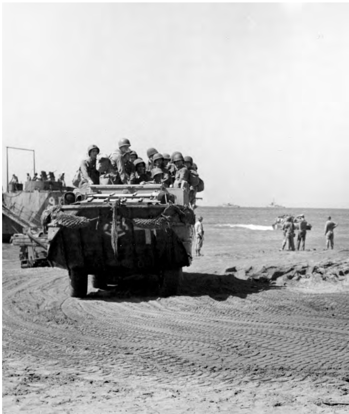
DUKW LANDING AT PAESTUM BEACH. These amphibian trucks brought light artillery and antitank guns ashore after the first assault waves had landed and, later in the day, brought men and supplies ashore.
