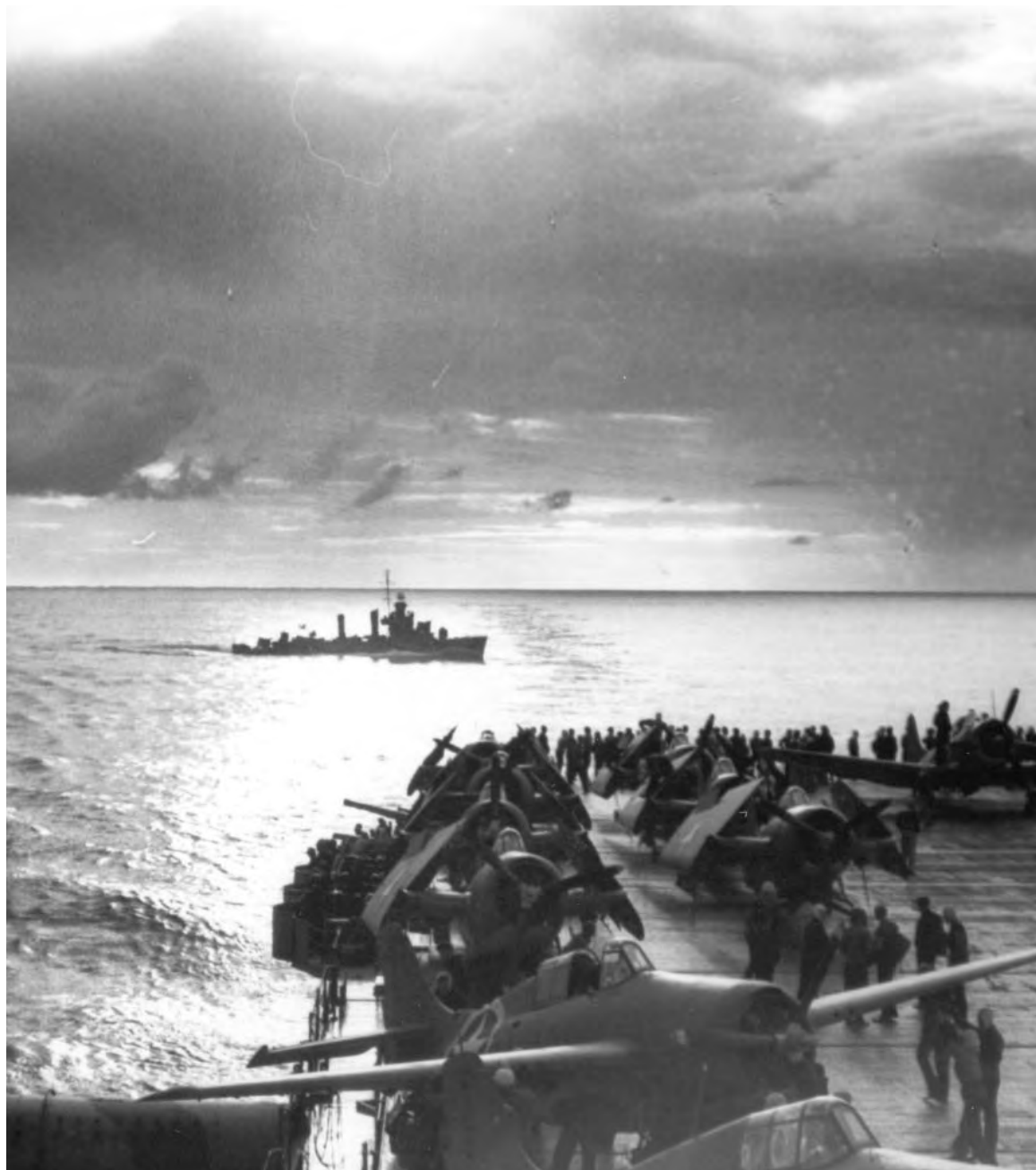
NAVY FIGHTER AIRCRAFT on flight deck of a carrier approaching the coast of North Africa. In the background is a destroyer escort. Two to four destroyers operated with each carrier, providing antisubmarine protection, picking up personnel from wrecked aircraft, and augmenting the antiaircraft screen around their charge. (Grumman F4F Wildcat, single seater, carrier fighters.)
