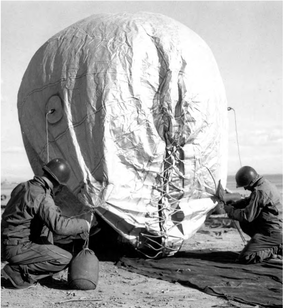
MEN WORKING ON A BARRAGE BALLOON. A number of balloons were used at the beachhead, chiefly in and around the port area. Floated at the end of a steel cable, their purpose was to prevent low-level strafing and dive-bombing attacks and to force the bombers high enough to give the antiaircraft gunners time to get on the target. Up to forty balloons were flown at one time over the port. These were filled with highly inflammable hydrogen gas, which was manufactured in the field. Helium gas was sometimes used but was harder to obtain.
