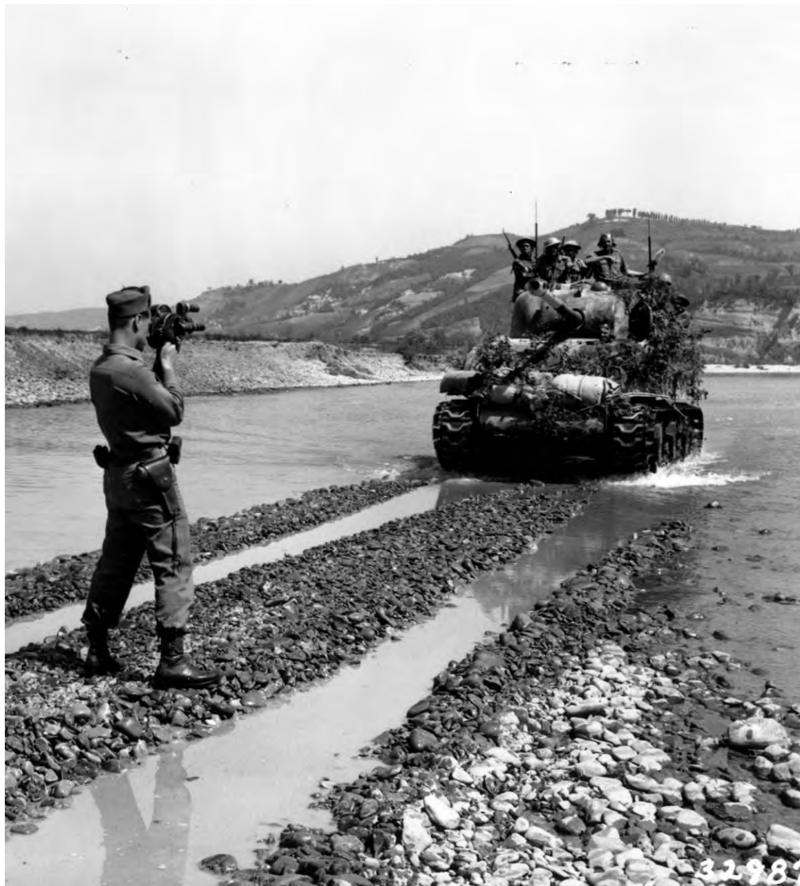
U. S. ARMY MOTION-PICTURE CAMERAMAN photographing the first tank of the South African armored force to cross the Reno River southwest of Bologna, 20 April. The practice of infantrymen riding on tanks while advancing was included in training for armored units in the United States early in 1944. (Sherman M4A3 tank with British 17-pounder; camera: PH-330 (Sig C), Eyemo, Bell, and Howell, 35-mm., three lenses mounted in turret.)
