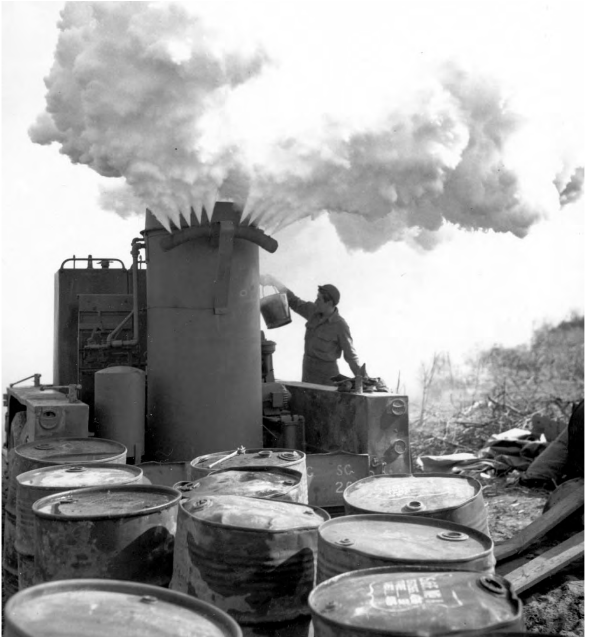
MECHANICAL SMOKE GENERATOR IN ACTION. Generators of this type were used at ports to prevent accurate bombing and in the field to conceal movements of troops. Large quantities of oil, about two 53-gallon drums per hour, were consumed. The generator was capable of converting hydrocarbon oils of low volatility into a fog of relatively great persistence. The special oil, usually referred to as fog oil and used for the generation of large area screens, was a petroleum by-product. The fog would frequently extend five miles or more downwind. (Smoke generator M1.)
