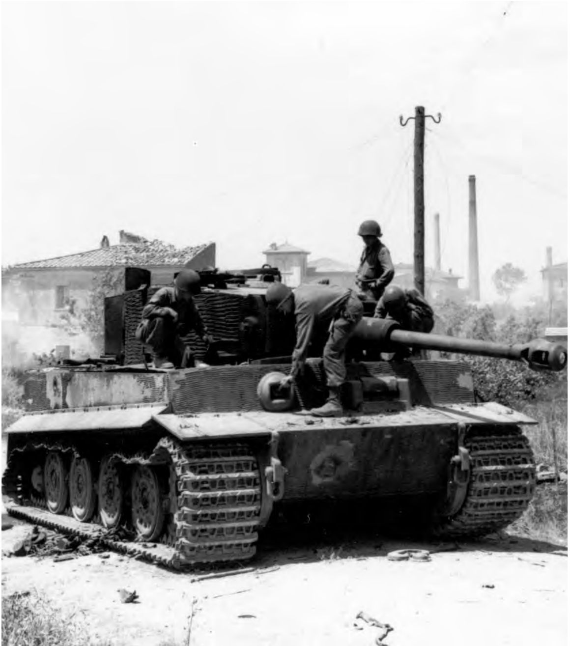
A TIGER TANK, such as was encountered in Tunisia and Sicily, but with a non-magnetic plastic coating. It is believed that most of the tanks thus coated were originally destined for the Russian front where the Germans were greatly troubled by delayed-action magnetic mines which were stuck onto the armor of their tanks by Russian infantry.
