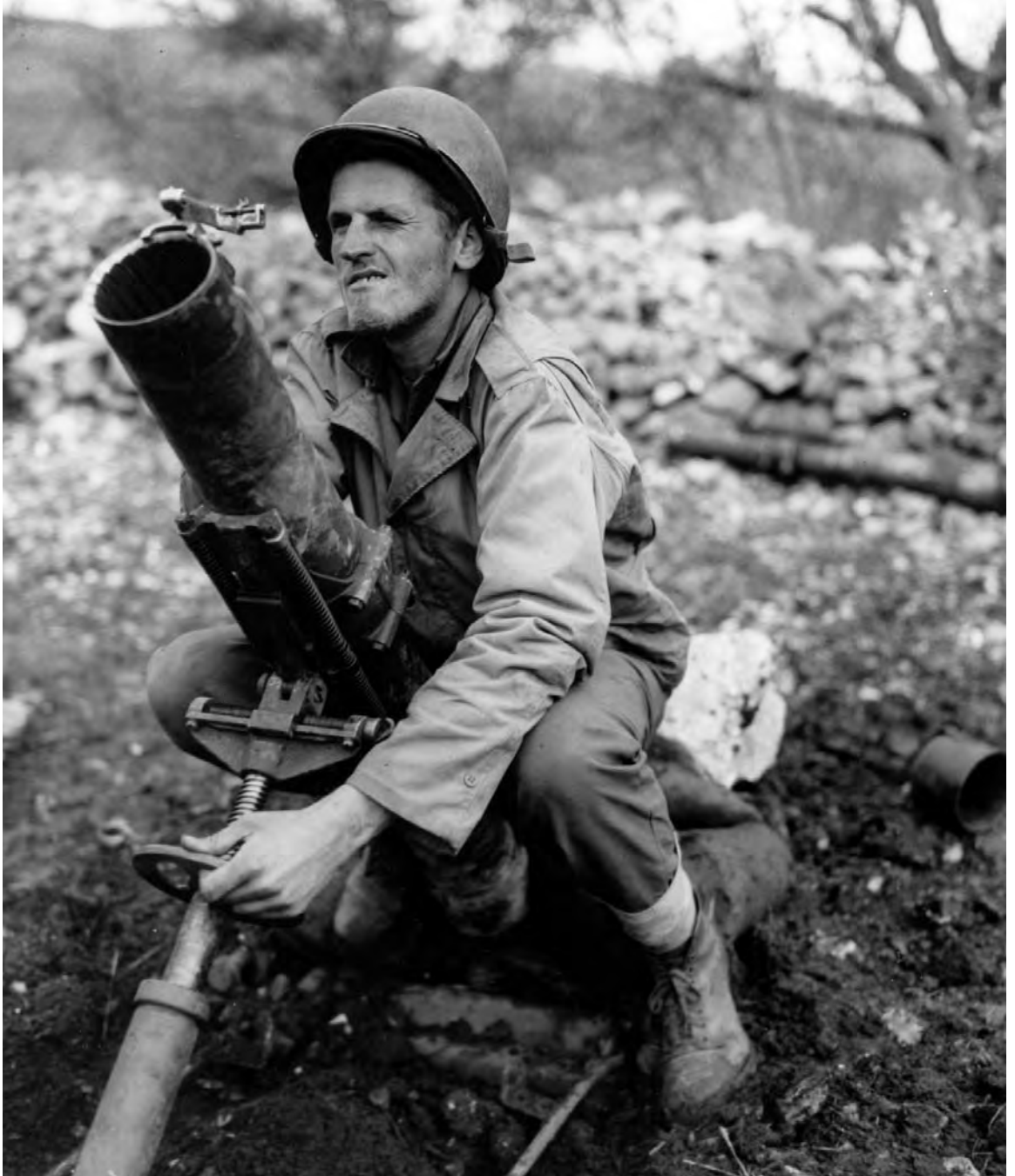
ADJUSTING ELEVATION AND DEFLECTION of 4.2-inch chemical mortar. This mortar had a rifled barrel and was designed for high-angle fire. Because of its accuracy (insured by rifled barrel), mobility, rate of fire, and ease of concealment, it was particularly suited for close support of attacking units.
