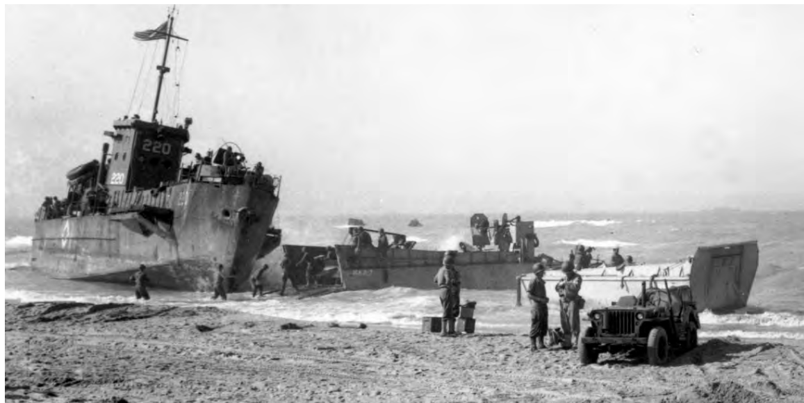
LANDING CRAFT ON BEACH. Top picture from left to right: LCI, LCM, and LCVP; on beach is a 1/4-ton 4 x 4 truck, jeep. Bottom picture: in middle distance is LST, with bow doors open, ramp down, and unloading onto a sectional ponton ramp; in the foreground are two LCT's. (The LCI (L) (1-350) was an infantry carrier with side ramps which could be lowered for unloading directly on the beach. It carried a crew of 3 officers and 21 men.)
