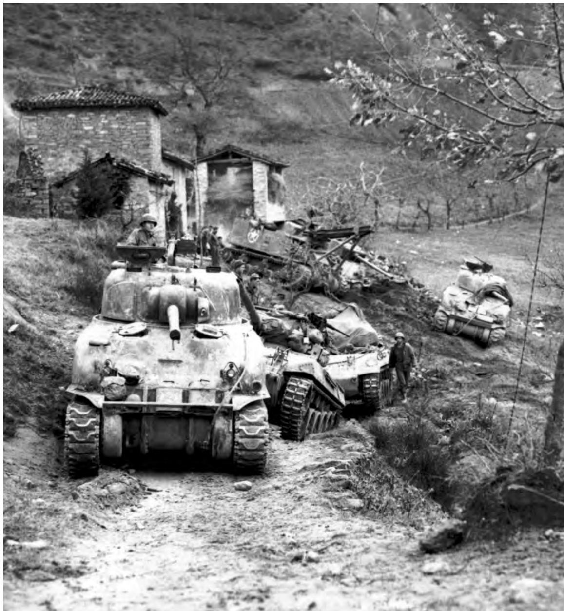
TANK MAINTENANCE POST in abandoned Italian farmhouse. During the long winter stalemate time was utilized to make major repairs on armored vehicles. Minor repairs, such as thrown tracks, were made at forward maintenance posts such as the above which was located only about 400 yards behind the front lines. (1, medium tank M4A1; 2 and 3, 76-mm. gun motor carriage M18; 4, medium tank M4A1; 5, medium tank M4, with 76-mm. gun (note different gun mount) : 6, tank recovery vehicle M31.)
