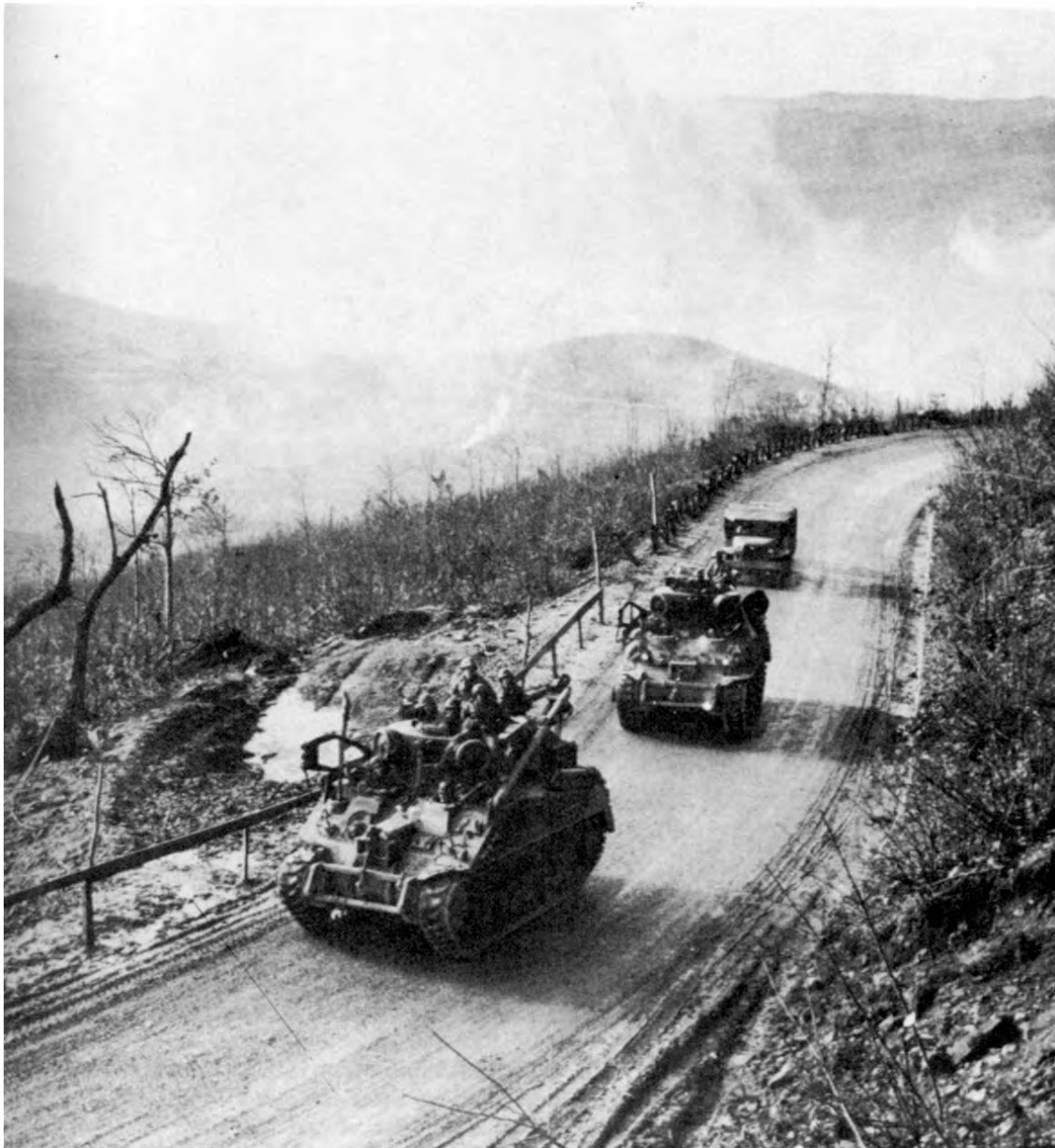
MOBILE FIELD ARTILLERY MAINTENANCE UNIT near the front. These units were used a great deal during the winter. Artillery off the main roads could be moved only with difficulty after the rains started and repairs that were normally made in shops behind the front had to be done in the field. The first two vehicles shown above are tank recovery vehicles M32, and are modifications of the M4 designed primarily for recovery of tanks from battlefields. The fixed turret replaces the customary tank turret. Third vehicle is weapons carrier, \frac{3}{4} -ton 4x4 truck.
