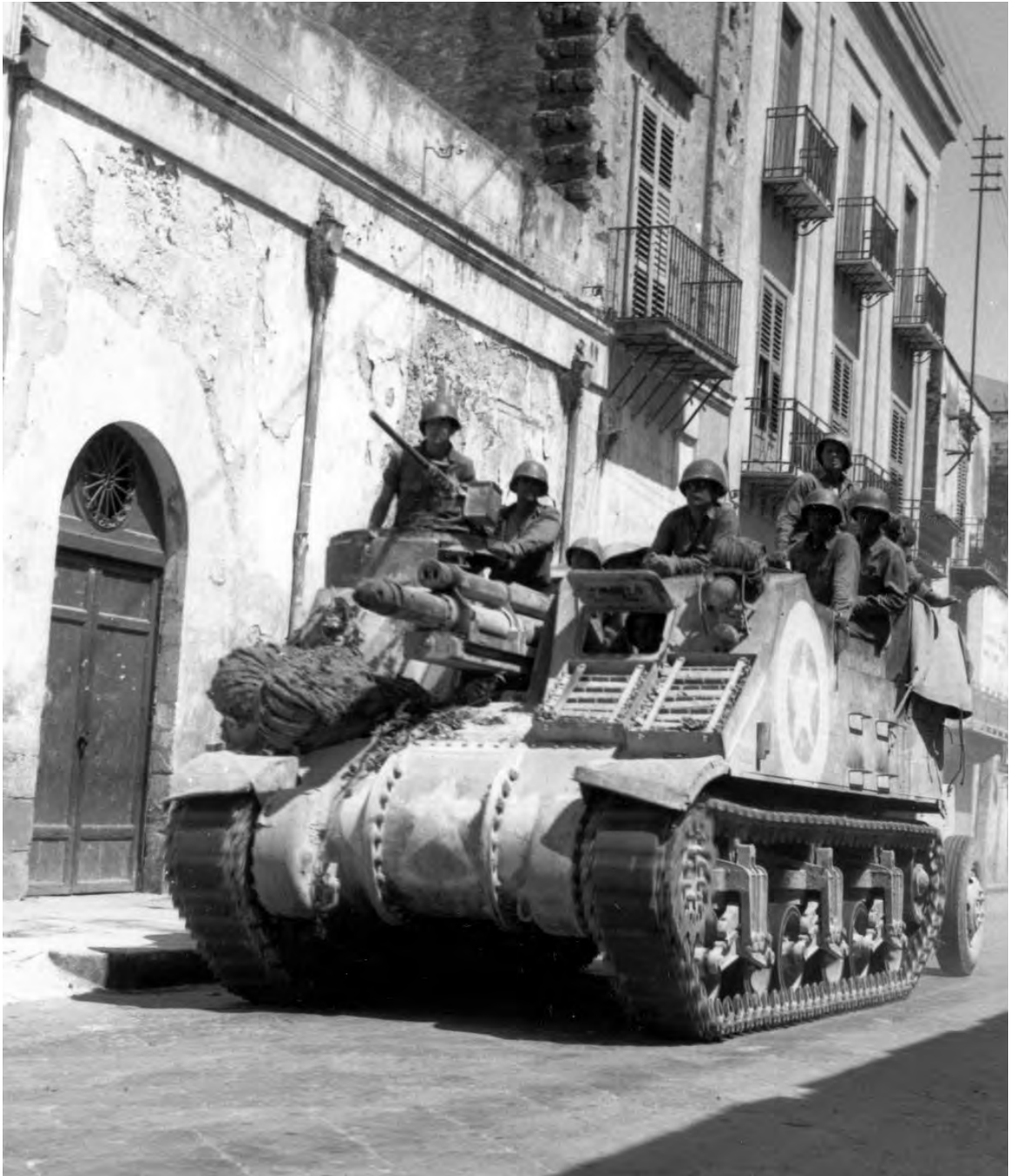
SELF-PROPELLED HOWITZER. This is the M7 howitzer motor carriage mounting a 105-mm. howitzer which was used for high angle as well as direct fire. The .50-caliber machine gun is mounted in a raised pulpit-like structure which gave the vehicle the nickname Priest. (Mounted on M3 tank chassis.)
