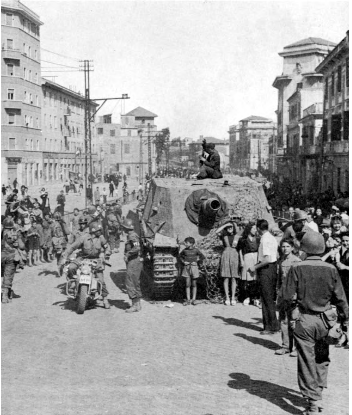
GERMAN GRIZZLY BEAR on a street in Rome. This is a close-support weapon and mounts a short-barreled howitzer in a high, armored superstructure (15-cm Stu. H. 43 on Pz. Kpfw. IV chassis.)
