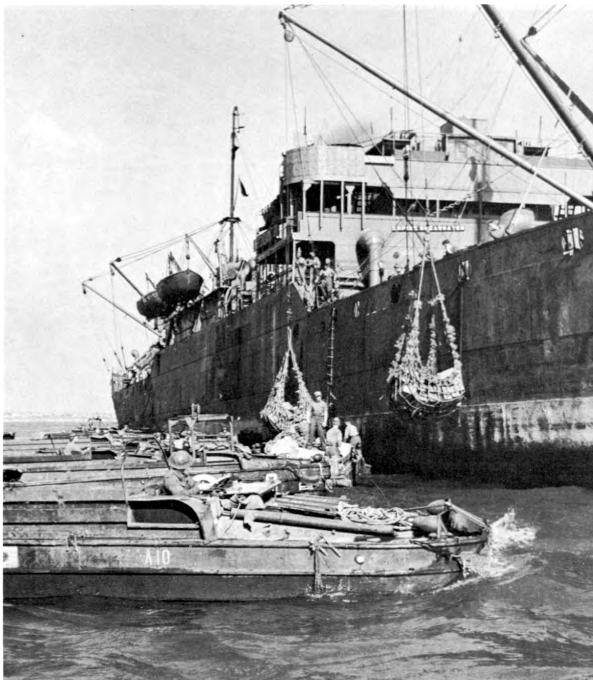
FREIGHTER UNLOADING CARGO INTO DUKW'S. Supplies for Anzio were carried by two methods: in truck-loaded LST's from Naples and in bulk-loaded Liberty ships or other freighters from Africa. After its capture, the port of Anzio sustained regular shelling by enemy artillery. The LST's docked at the port and the freighters unloaded into smaller craft or DUKW's offshore.
