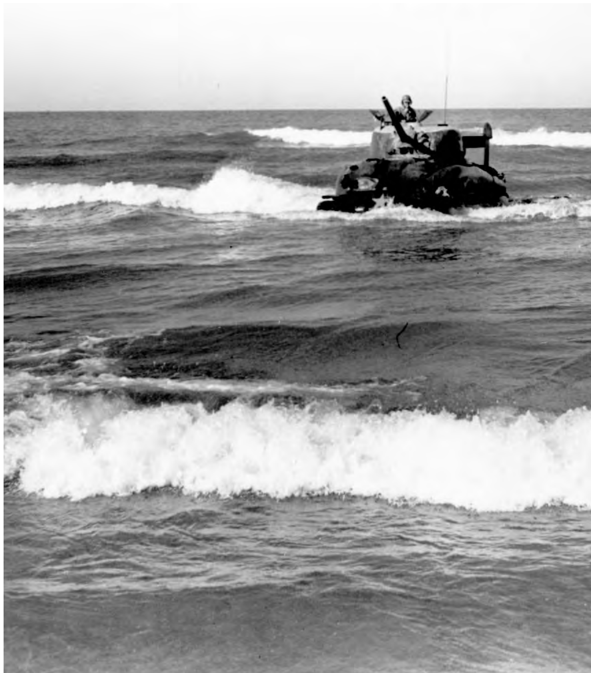
TESTING A WATERPROOFED SHERMAN TANK on an African beach. These tanks were intended to go, during an assault, onto the beach with the infantry whenever possible. The main body of tanks would follow on LST's as soon as the beach-head had been secured. The follow-up tanks, landed from the ship via ponton piers directly to shore, were not normally waterproofed. (Sherman tank M4A1.)
