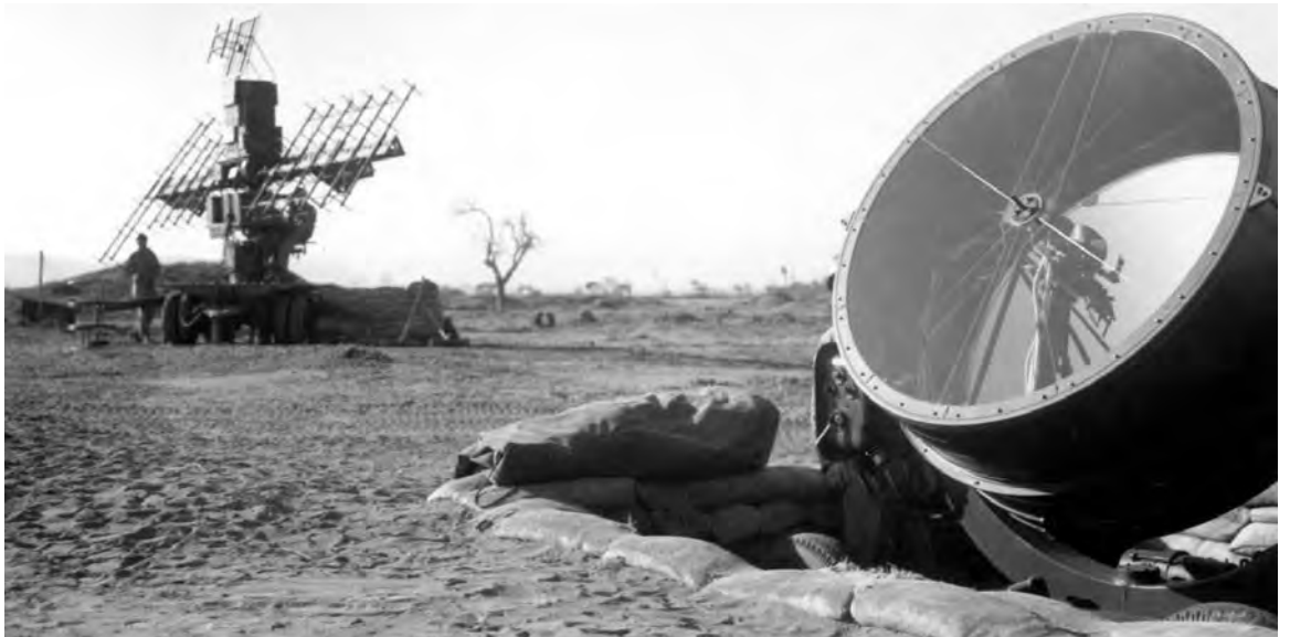
RADAR SETS NEAR CASABLANCA. This type of set was part of the equipment of the invading forces. By the end of December 1942, fifteen of these units were in operation as part of the air warning system of Casablanca. The searchlight automatically followed planes tracked by the radar. The city was almost at the maximum range of enemy bombers and was the target for few raids. (Radar set SCR 268.)
