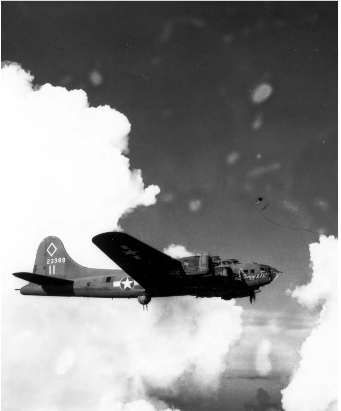
HEAVY BOMBER, FLYING FORTRESS. This and the B-24 were the two heavy U. S. four-engined bombers used in the Mediterranean area. (Boeing B-17.)
