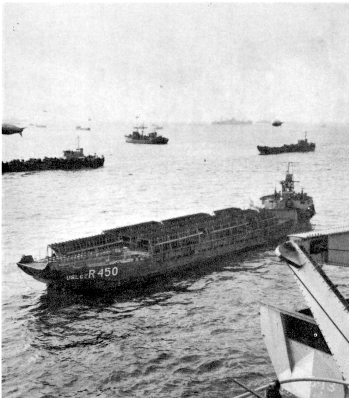
ROCKET SHIP CONVERTED FROM AN LCT. Ahead of the first wave of assault troops in landing craft were rocket ships mounting tiers of rocket launchers. As these drew within range of the beach defenses they discharged their rockets. The first troops landed immediately afterward. Rocket ships were equipped with launchers for up to 1,000 rockets.
