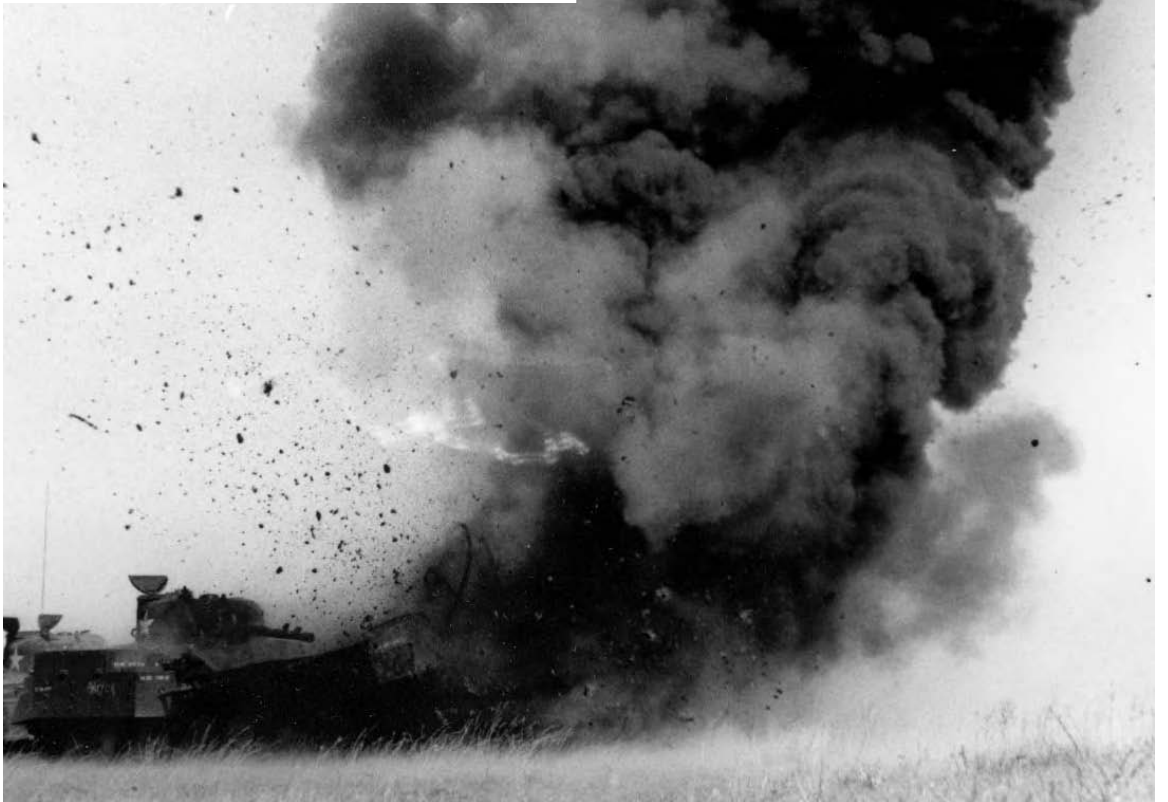
SHERMAN TANK WITH "SCORPION" ATTACHMENT, detonating mines during a test. The Scorpion was a revolving drum with chains attached (insert); when in motion it acted as a flail and could clear a path through a mine field for infantry and other tanks to follow. It was developed by the British and used extensively by them in desert warfare.
