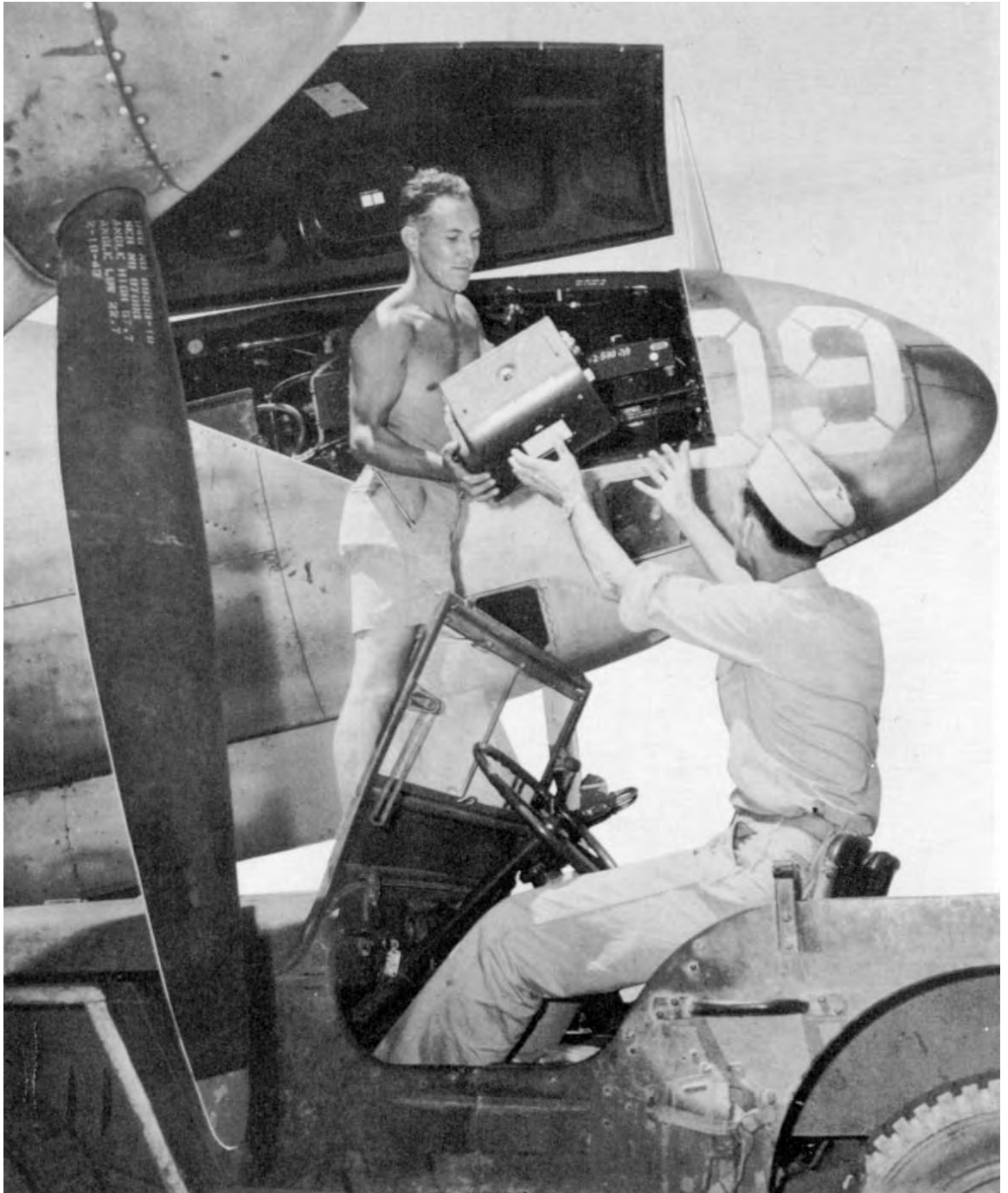
REMOVING FILM FROM FIGHTER PLANE after a reconnaissance flight. This long-range plane was adapted for photographic work by removing the armament and installing camera equipment instead. (P-38.)
