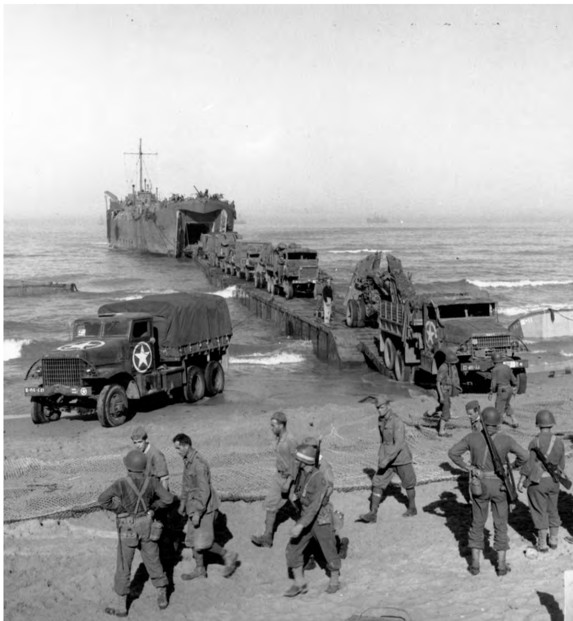
A BATTERY OF ANTI-AIRCRAFT GUNS being unloaded from an LST, the largest type landing craft used during the operation. The prototype of the landing ship, tank, was built by the British and used in the invasion of North Africa. The LST shown is a seagoing ship. Its payload was from 1,600 to 1,900 tons of which 400 tons were deck-loaded. The ship could carry on each side sectional ponton ramps for inaccessible landings (in use above). The first three vehicles are 6-ton 6 x 6 prime mover trucks. (90-mm. guns.)
