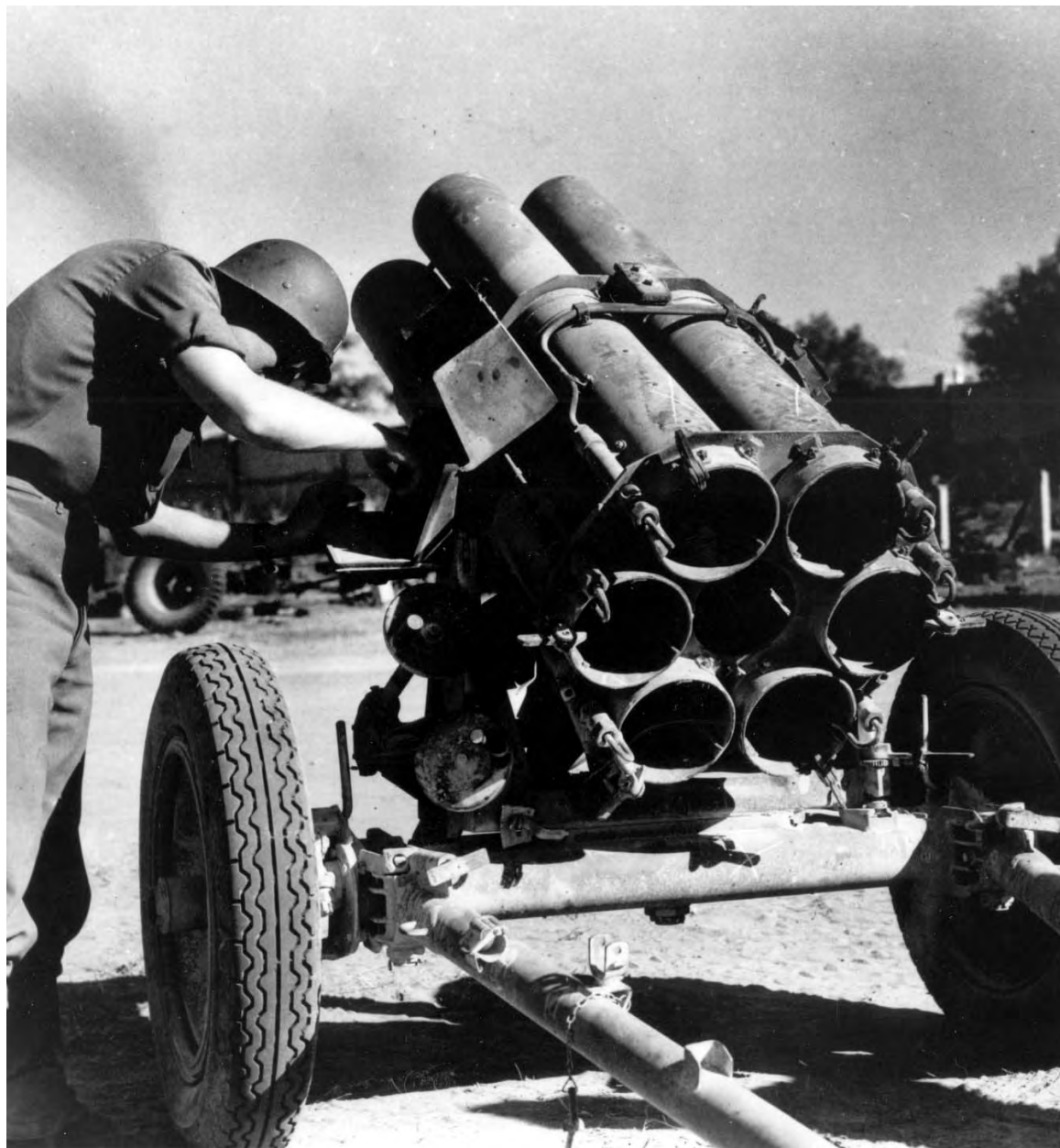
GERMAN SIX-BARRELED ROCKET LAUNCHER. This weapon fired high-explosive, incendiary or smoke rockets and was light enough to be moved with ease. The screaming sound of the rockets had an adverse psychological effect on troops at the receiving end and the rockets were nicknamed "screaming meemies." Artillery sound-ranging equipment could not locate the rocket launchers because firing did not cause a report. The enemy used this type of weapon until the end of the war. (15-cm. Nebelwerfer , 41.)
