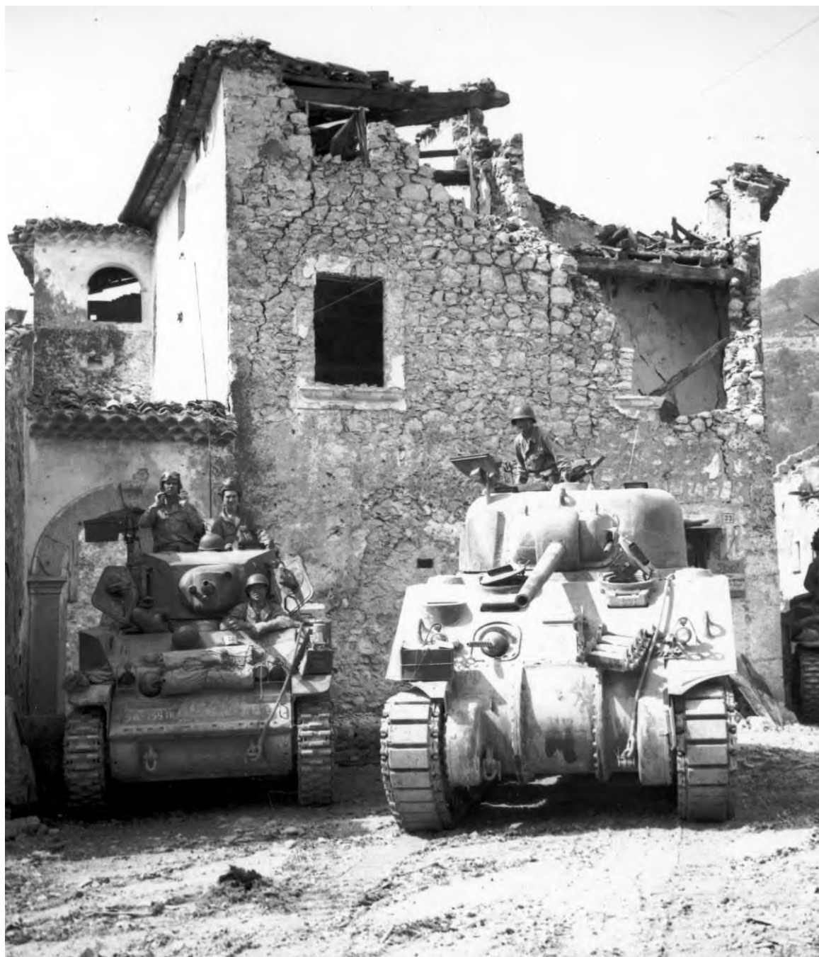
U. S. TANKS IN CORENO AUSONIO on 14 May. The same tanks, manned by Americans, were attached to the French mountain troops making a drive from the Castelforte area on the right flank of the Fifth Army, through the Aurunci Mountains and into the Liri Valley. (Left, light tank M5; right, medium tank M4.)
