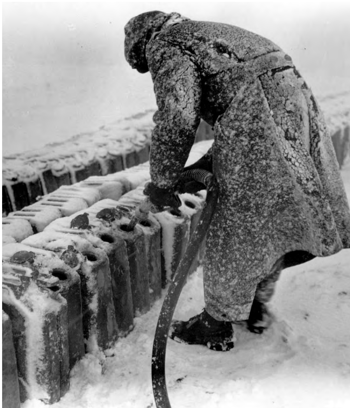
FILLING CANS WITH GASOLINE at the Raticosa Pass on Highway 65, terminal of the pipeline from Leghorn. These cans were picked up by truck and distributed to individual units. As the front moved, the pipeline was extended to keep up with the troops. (Five-gallon gasoline cans.)
