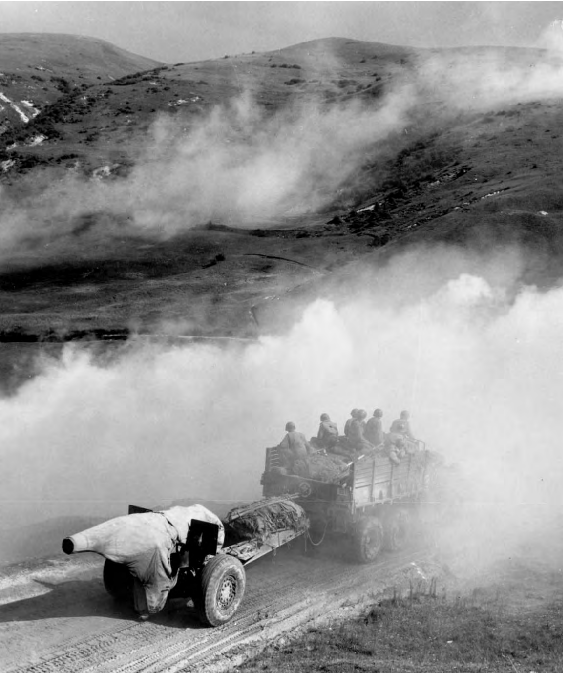
TRUCK TOWING HOWITZER along Highway 65 during the beginning of the 1 October drive. Smoke is from M2 smoke generators. (6-ton truck; 155-mm. howitzer.)
