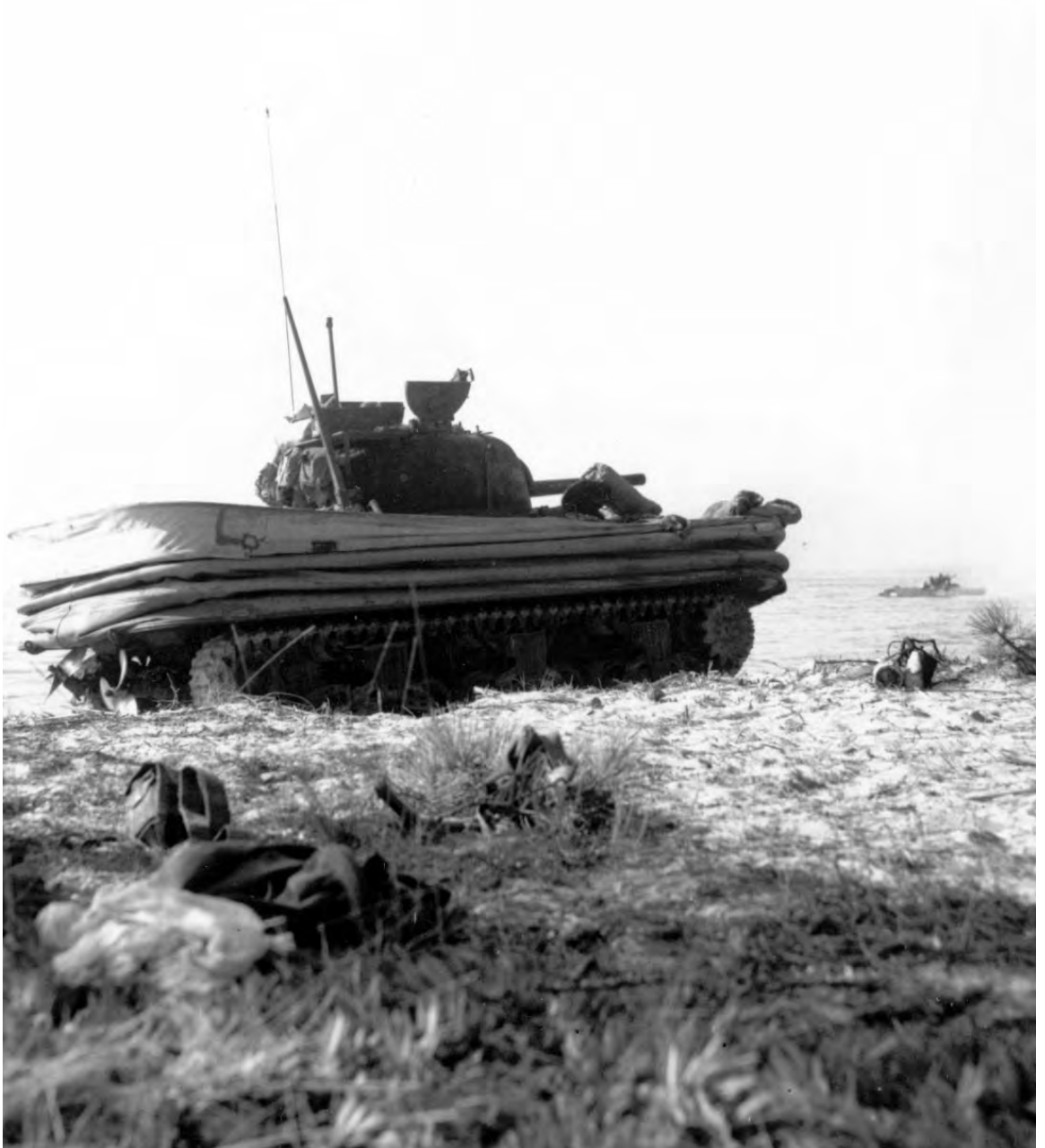
DUPLEX-DRIVE TANK. Amphibian tanks were launched from LCT's about 2,000 yards offshore to support infantry on the Saint-Tropez peninsula assault. By means of the duplex drive a regular medium tank was converted into an amphibian. When the canvas screen was raised and held in place by mechanical means the tank floated. The DD tank was vulnerable to mines and underwater obstacles. Offshore at right an amphibian 2 1 / 2 -ton truck is bringing a 105-mm. howitzer to the beach.
