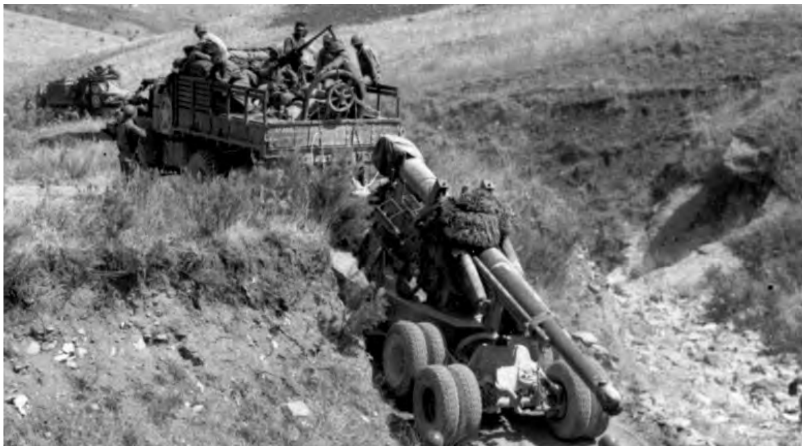
THE LONG TOM. This was the largest U. S. piece of artillery in Sicily. A 7 1 / 2 -ton 6 x 6 prime mover truck towing a gun into position (top). Firing from a camouflaged position in an orchard (bottom). (155-mm. gun with standard carriage.)
