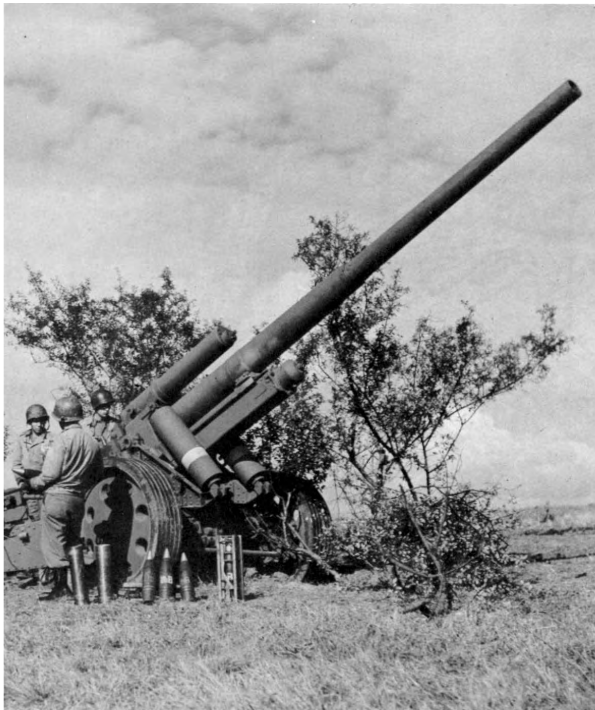
CAPTURED GERMAN ARTILLERY. The standard medium gun of the German Army. It was a World War I model which was used on all German fronts and was part of the corps artillery. The caliber was 10-cm.
